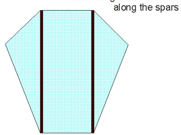
fold the tape 30mm on back side at each end
